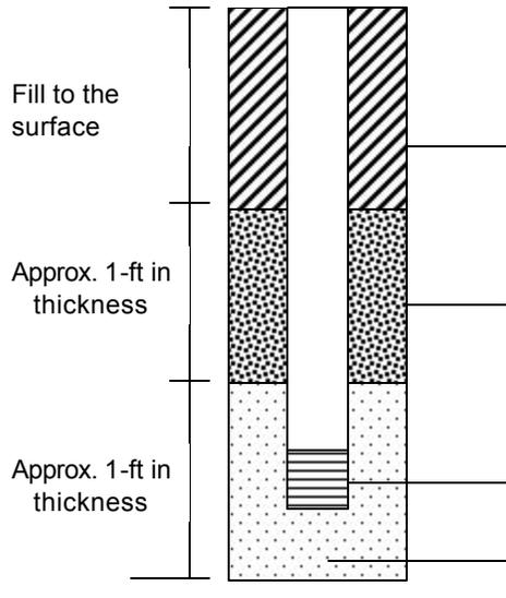
**Figure 2 – Multi-depth Gas Probe Construction Diagram**
